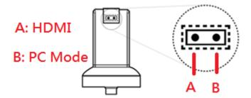
If you connect to HDMI monitor, please press HDMI button (A) to switch to correct mode.
